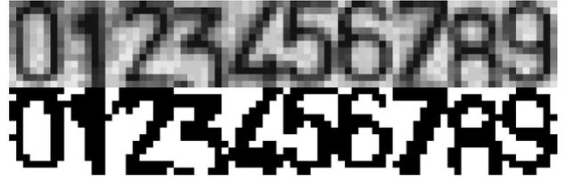
Fig. 1. (top) original grey-scale images of car plates digits and (bottom) preprocessed patterns.
